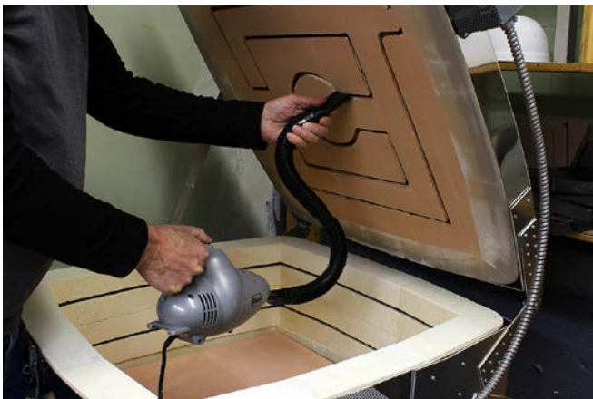
Vacuuming out lid element groves
